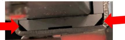
**7.** Mount the new sliding plate with wax. The track with the wax must be up against the sliding rail and outwards, towards the arm so to say.
