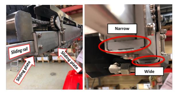
5. Remove the screws on one sliding plate first. Make sure that you don't lose any spring washers. If
