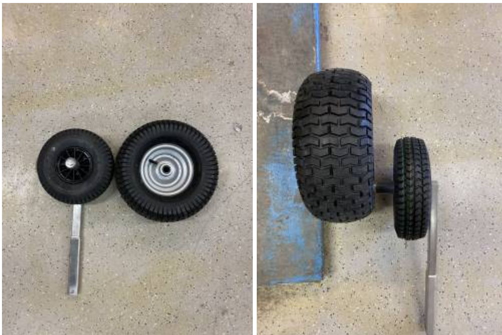
High wheels compared to the standard wheels.
