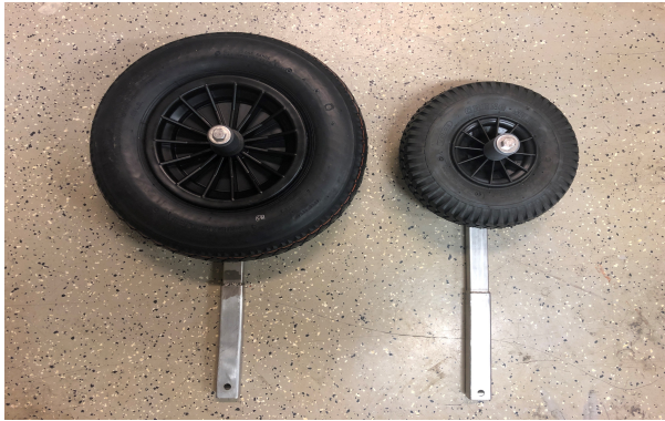
Wide wheels compared to the standard wheels.
