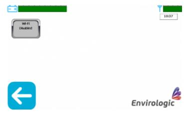
**Step 5.** When the button change color to green and says "Wi-Fi enabled" the robot will search for nearby Wi-Fi's. The robot will list the three strongest signals.
