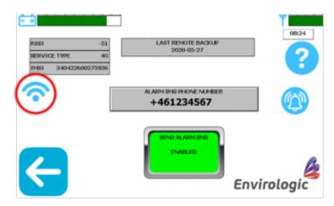
Step 4. Press the "Wi-Fi disabled" -button to enable Wi-Fi.
