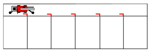
Markers are magnetic and the robot has a magnetic sensor to read the markers. The magnetic markers are only placed in the aisle during the automatic wash. Brackets are mounted permanently. The magnetic sensor must be within 10 cm from the markers, otherwise the sensor cannot read the markers.
