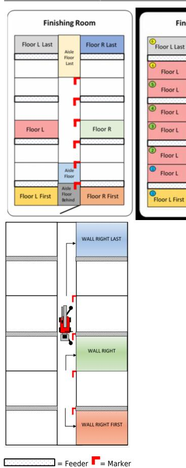
**"Floor L"** and **"Floor R"** could, for example, be programmed at marker 3 and then applied to marker 1,2,3,4, 5 and 6 because there are similar boxes there. The boxes are mirror-flipped but only with the feeders on the other side so same program can be applied in these, just have that in mind during the
