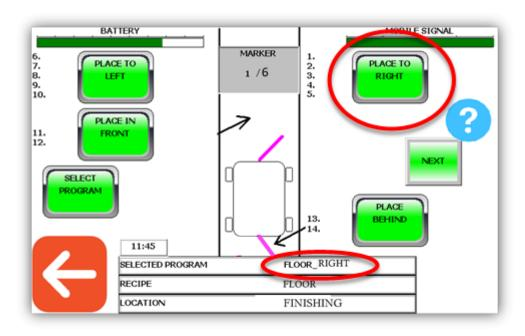
Programs created for the right side are placed at the right side (position 1 - 5 as shown on the screen). Programs created for the left side are placed at the left side (positions 6 - 10).
