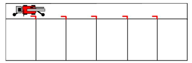
Markers are magnetic and the robot has a magnetic sensor to read the markers. The magnetic markers are only placed in the aisle during the automatic wash. Brackets are mounted permanently. The magnetic sensor must be within 10 cm from the markers, otherwise the sensor cannot read the markers.
