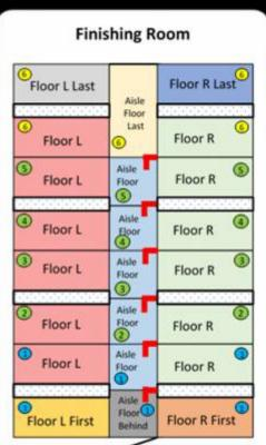
**"Floor L"** and **"Floor R"** could, for example, be programmed at marker 3 and then applied to marker 1,2,3,4, 5 and 6 because there are similar boxes there. The boxes are mirror-flipped but only with the feeders on the other side so same program can be applied in these, just have that in mind during the
