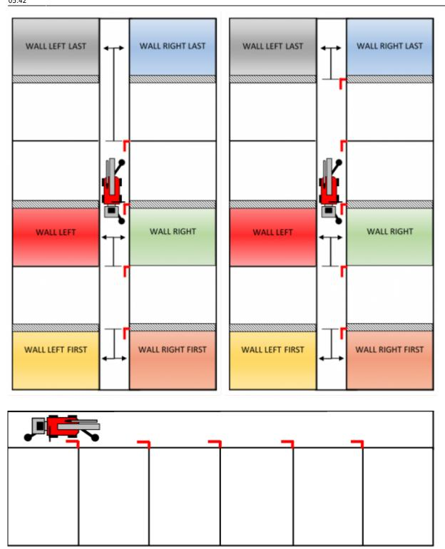
Markers are magnetic and the robot has a magnetic sensor to read the markers. The magnetic markers are only placed in the aisle during the automatic wash. Brackets are mounted permanently. The magnetic sensor must be within 10 cm from the markers, otherwise the sensor cannot read the markers.
