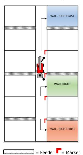
**"Floor L"** and **"Floor R"** could, for example, be programmed at marker 3 and then applied to marker 1,2,3,4, 5 and 6 because there are similar boxes there. The boxes are mirror-flipped but only with the feeders on the other side so same program can be applied in these, just have that in mind during the programming so you keep same distance on both sides.
