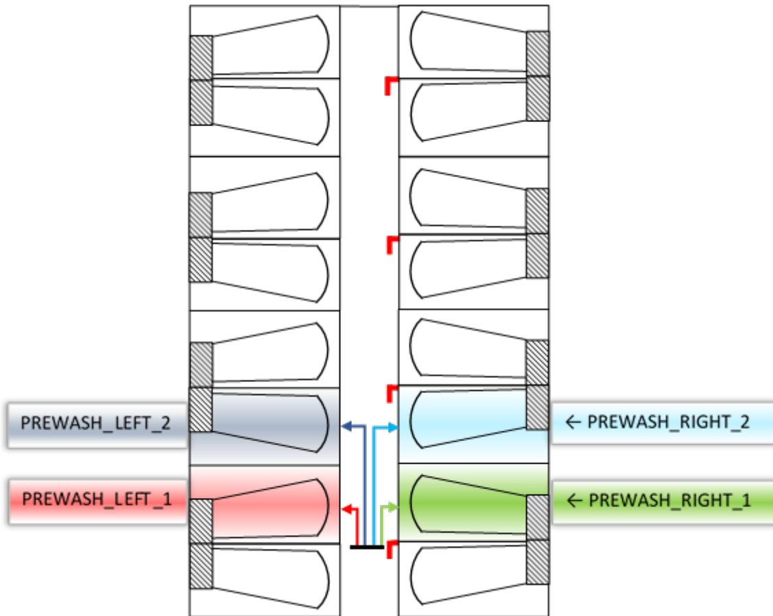
Markers are magnetic and the robot has a [magnetic sensor](#) to read the markers. The magnetic markers are only placed in the aisle during the automatic wash. Brackets are mounted permanently. The magnetic sensor must be within 10 cm from the markers, otherwise the sensor cannot read the markers.
