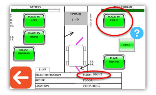
Programs created for the right side are placed at the right side (position 1 - 5 as shown on the screen). Programs created for the left side are placed at the left side (positions 6 - 10).
