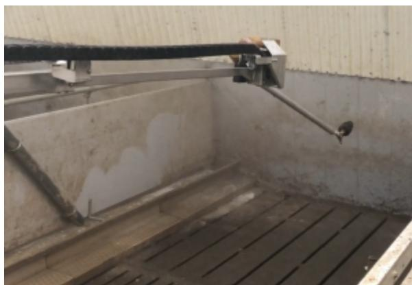
4. Make a movement with the boom or tower that lasts for 5 seconds without water on. This will give the steel ball time to fall down and block the other nozzle.
