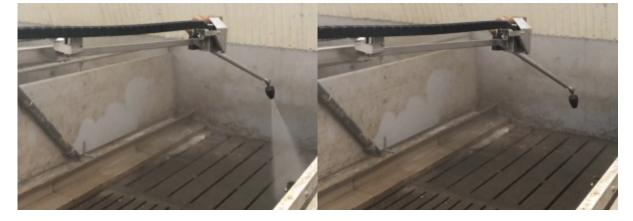
2. Rotate (if necessary) the nozzle so the correct nozzle is placed straight down. You might have to adjust the arm position as well (arm position should be approx. 45 degrees or 135 degrees out from the boom).
