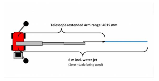
It's very important to program the robot correctly if you robot is equpped with a double nozzle. If not, there may come water from the wrong nozzle.
