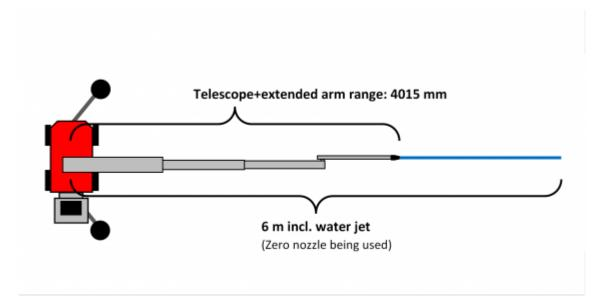
It's very important to program the robot correctly if you robot is equipped with a double nozzle. If not, there may come water from the wrong nozzle.
