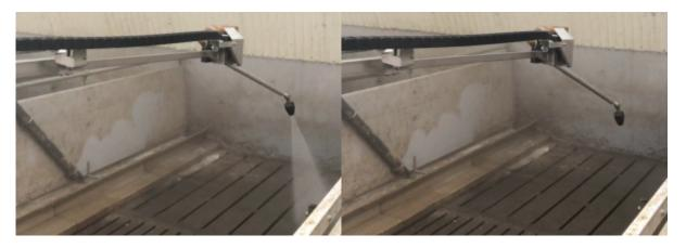
2. Rotate (if necessary) the nozzle so the correct nozzle is placed straight down. You might have to adjust the arm position as well (arm position should be approx. 45 degrees or 135 degrees out from the boom).
