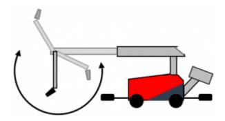
The arm starts from its parked position parallel to the boom (position about -55). The arm can go out about 315°(to position 1100), so it points towards the ceiling.
