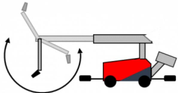
The arm starts from its parked position parallel to the boom (position about -55). The arm can go out about 315° (to position 1100), so it points towards the ceiling.
