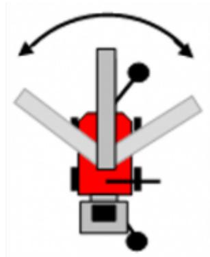
The tower can go about 200° in both directions (positions  $\pm 1000$ ) from its parked forward position (about position 0).
