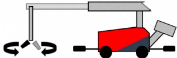
The nozzle can spin 360° in both directions. The nozzle is parked when the arm is parked and nozzle points downwards.
