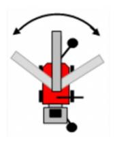
The tower can go about  $200^{\circ}$  in both directions (positions  $\pm 1000$ ) from its parked forward position (about position 0).
