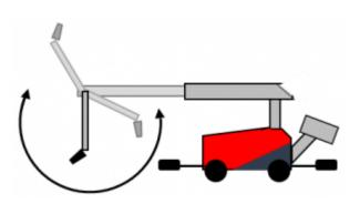
The arm starts from its parked position parallel to the boom (position about -55). The arm can go out about 315°(to position 1100), so it points towards the ceiling.
