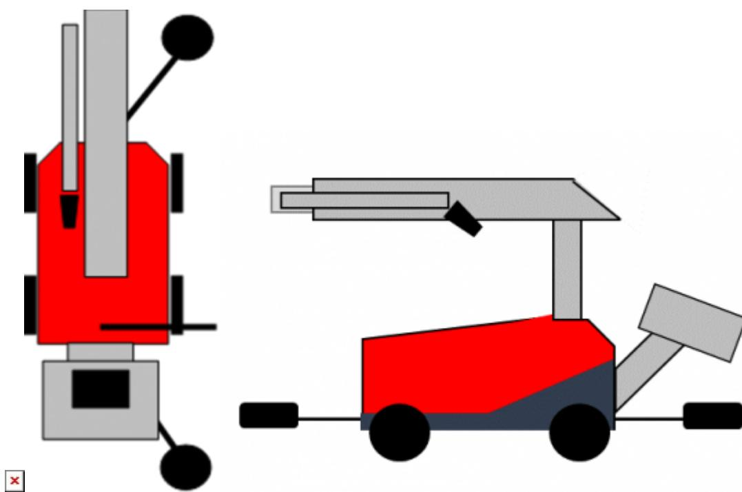
Keep these positions in mind when the automatic wash starts, and the robot makes its first automatic parking after it has sensed the first marker. Does the robot set as above? The robot also parks after a program is finished.
