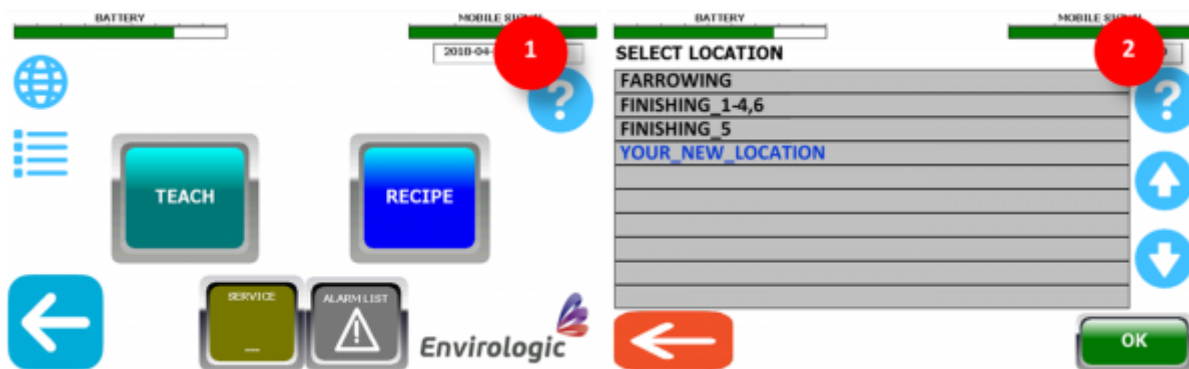
Picture 3: You can now choose whether you want to create a new recipe (step 1.) or edit an existing recipe (step 2.).
