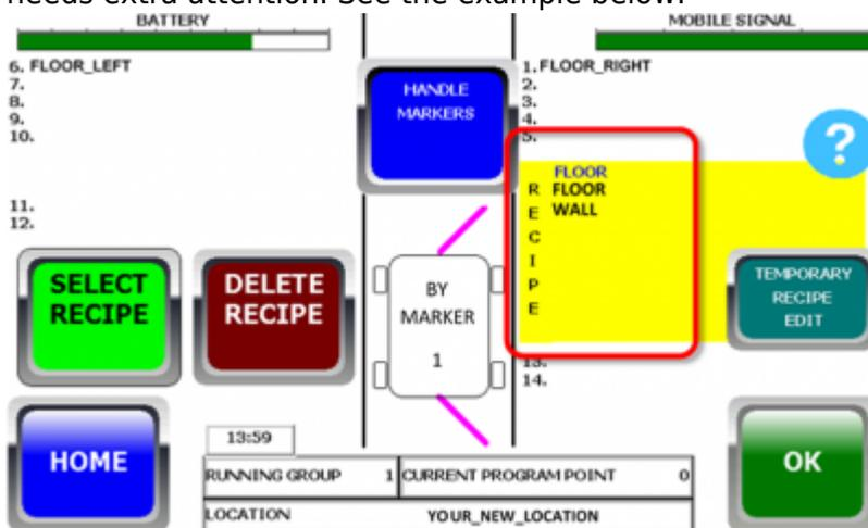
Make sure that the robot is positioned with the marker sensor in front of the first marker (up to 100 cm in front) before you press "OK". When you press the "OK"-button the robot will run forward to find the marker and start the automatic wash based on the recipe queue you have selected.
