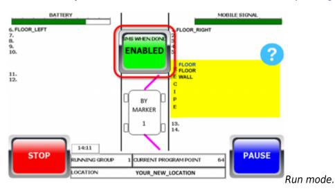
• If you press "**STOP**" during an active wash, the robot will finish the program it has started and stop when the program has ended.
