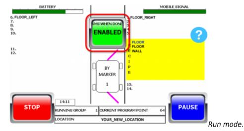
• If you press "STOP" during an active wash, the robot will finish the program it has started and stop when the program has ended.
