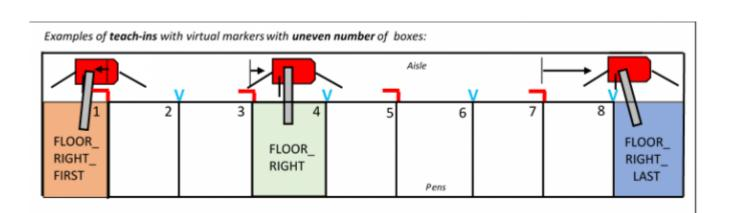
Since the program for the last pen is learned from marker 7 (last physical marker), this program must also be placed at marker 7 in the recipe.
