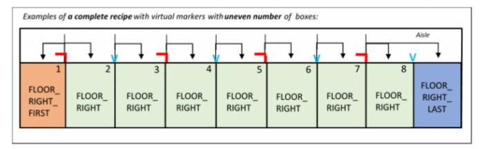
If there are identical boxes, you can place same program for each of these markers. A program from a physical marker can also wash from a virtual marker. Notice that marker 8 is without programs in these examples. It's very important to understand how the robot will move for each program. Is it possible to use the last virtual marker in the recipe?
