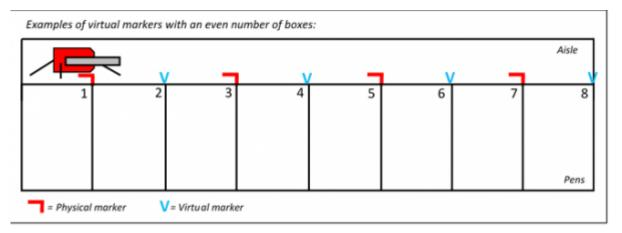
In this example, there are 4 physical markers in every other position. Between these, 3 virtual markers are created where otherwise there would have been physical markers. As mentioned in the text above, a virtual marker is also created after the last physical marker and in this example, it ends up in the wall. So, the last marker will not be used in the recipe build-up, so you shouldn't place any programs at marker 8 in this example.
