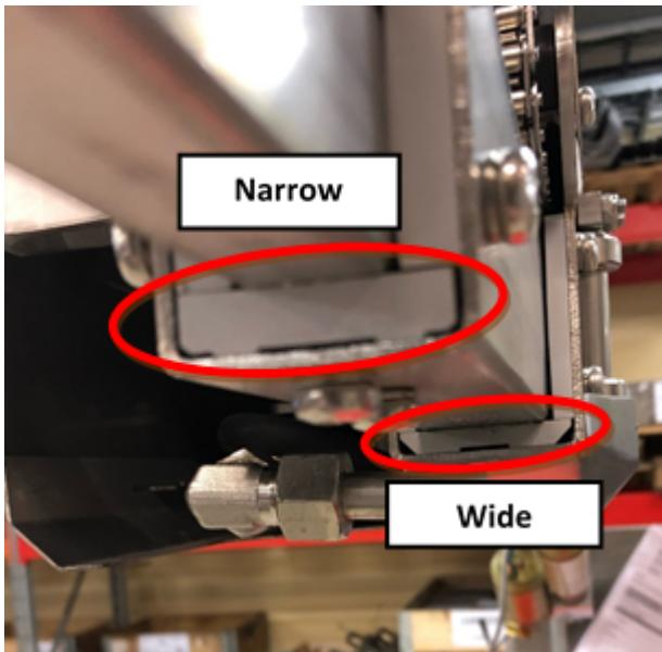
**5.** Remove the screws on one sliding plate first. Make sure that you don't lose any spring
