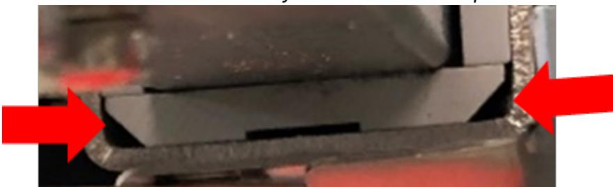
**7.** Mount the new sliding plate with wax. The track with the wax must be up against the sliding rail and outwards, towards the arm so to say.
