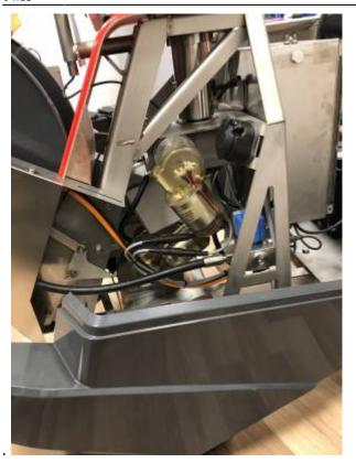
**3.** Dismount the 10mm hexagon screw like the picture below, and pull the plunge out.
