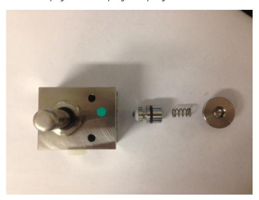
**8.** Pull a straw from a steel-brush (or similar) into the small hole in the center of the plunge until you can see the straw in the other hole shown in the picture. Make sure you have good lighting when doing this.
