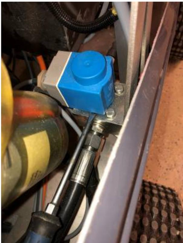
3. Unscrew the hose connected to the 90 degrees bend.
