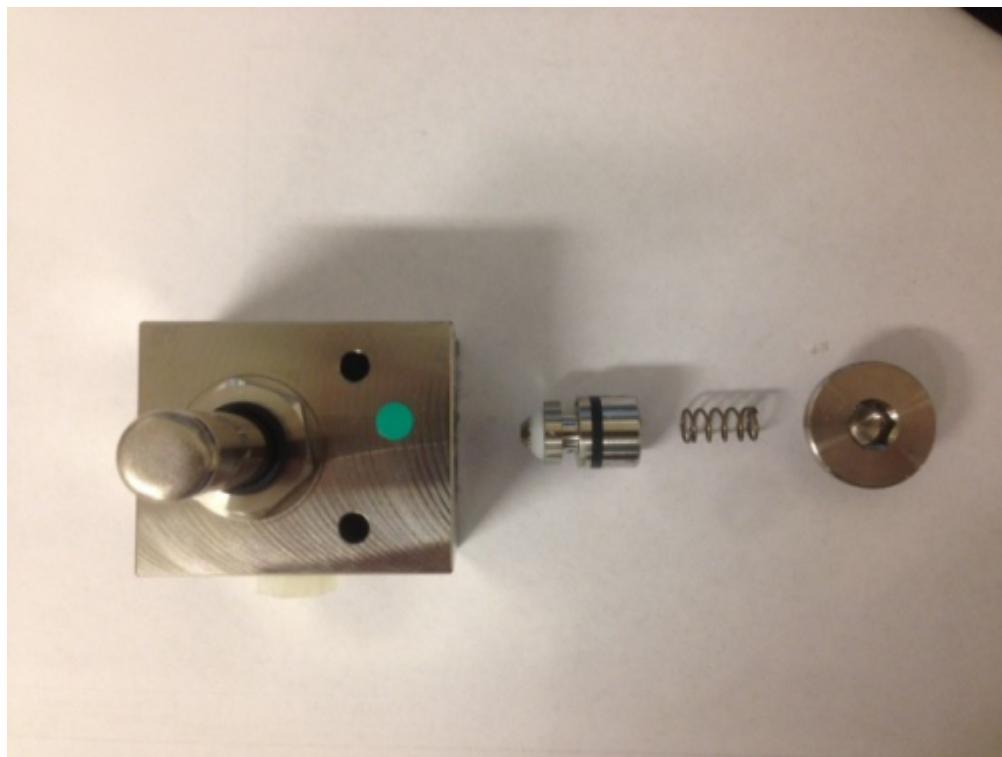
**8.** Pull a straw from a steel-brush (or similar) into the small hole in the center of the plunge until you can see the straw in the other hole shown in the picture. Make sure you have good lighting when doing this.
