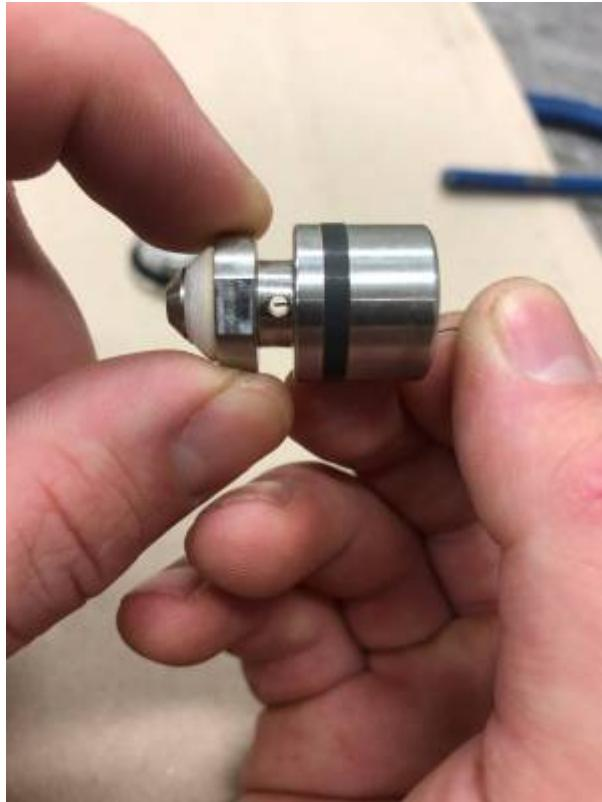
**9.** Rinse with water or blow with compressed air.
