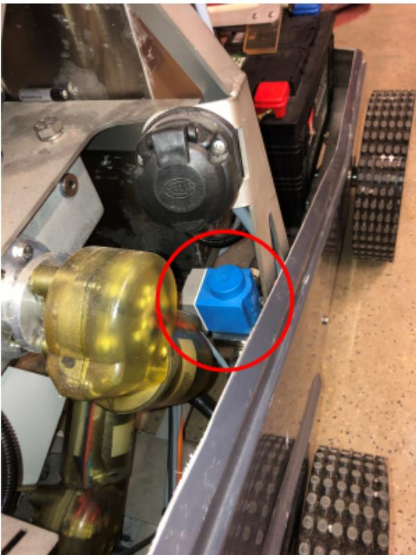
2. Snap the coil off with a screwdriver like in the picture below.
