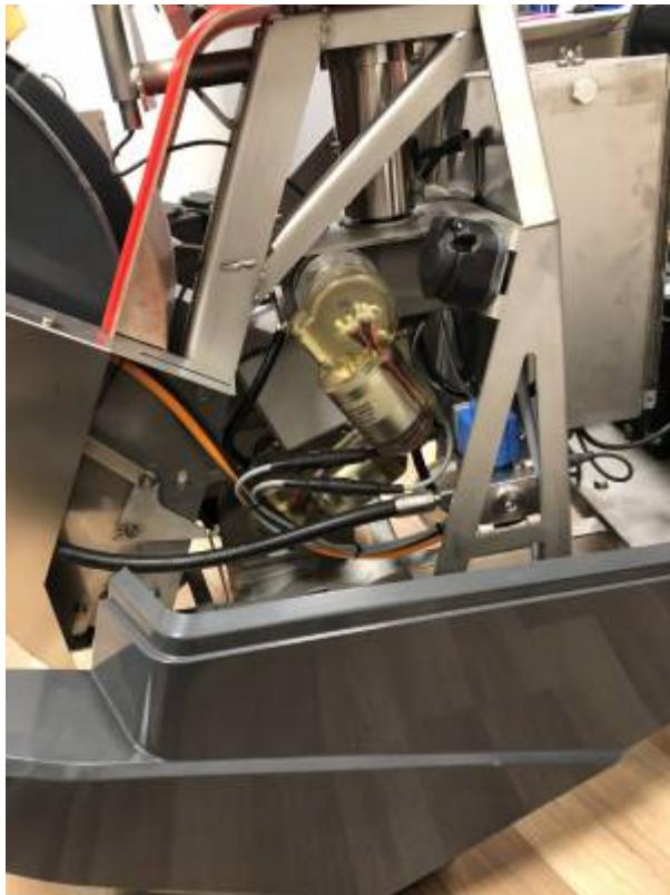
**3.** Dismount the 10mm hexagon screw like the picture below, and pull the plunge out.
