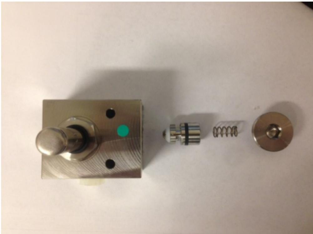
**4.** Pull a straw from a steel-brush (or similar) and push it into the small hole in the center of the plunge until you can see the straw in the other hole shown in the picture below.
