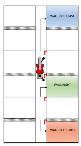
= Feeder = Marker "Floor L" and "Floor R" could, for example, be programmed at marker 3 and then applied to marker 1,2,3,4, 5 and 6 because there are similar boxes there. The boxes are mirror-flipped but only with the feeders on the other side so same program can be applied in these, just have that in mind during the programming so you keep same distance on both sides.
