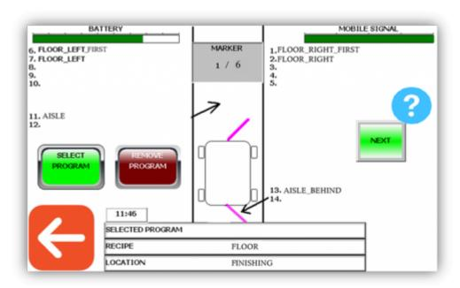
This picture shows how it would look like at marker one with all programs according to the examples at the previous sheet. The location is named Finishing. Recipe is named Floor. The location has 6 markers. The
