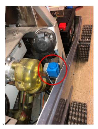
**2.** Unscrew the grey plastic side on the robot to get access to the 10mm hexagon screw.
