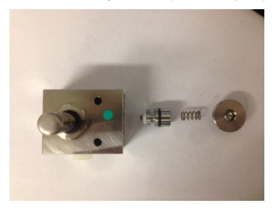
**4.** Pull a straw from a steel-brush (or similar) and push it into the small hole in the center of the plunge until you can see the straw in the other hole shown in the picture below.
