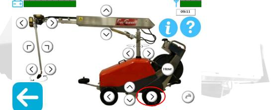
2. If the hose spreader is not moving, wait for at least 2 minutes, the hose spreader can stand and wait at its turning point before turning. If it does not start, then the troubleshooting begins in the hose spreaders enclosure.
