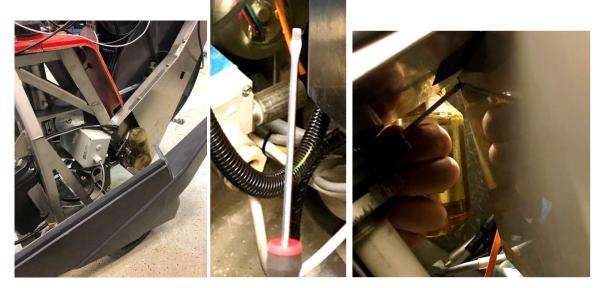
**4.** Due to vibrations in the robot, the connectors may jump of its place. To fix this we put a small amount of MS Polymer on the connector to hold it in place
