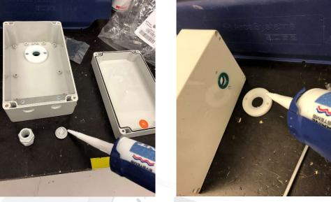
**Note:** Every robot that needs repair done inside the hose spreaders enclosure, needs to be sealed with MS Polymer in the three different entrances if it is not already done.
