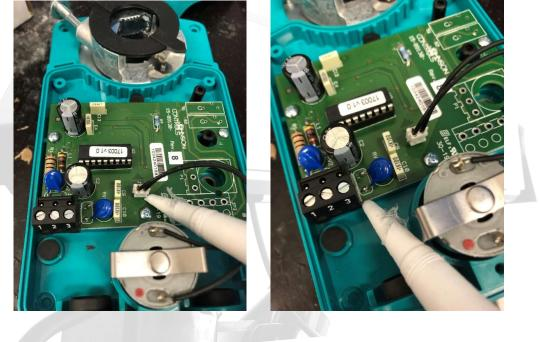
Envirologic AB Söderforsgatan 1 SE-752 28 Uppsala tel. +46 18 39 82 30 E-mail: <u>service@envirologic.se</u> www.envirologic.se 5. Measure on the connector if you have power from the circuit board, between pins 1 and 2 it should be 24 V when the spreader motor is running. When the motor is going the opposite direction, it will have 24V between pin 1 and pin 3 too
